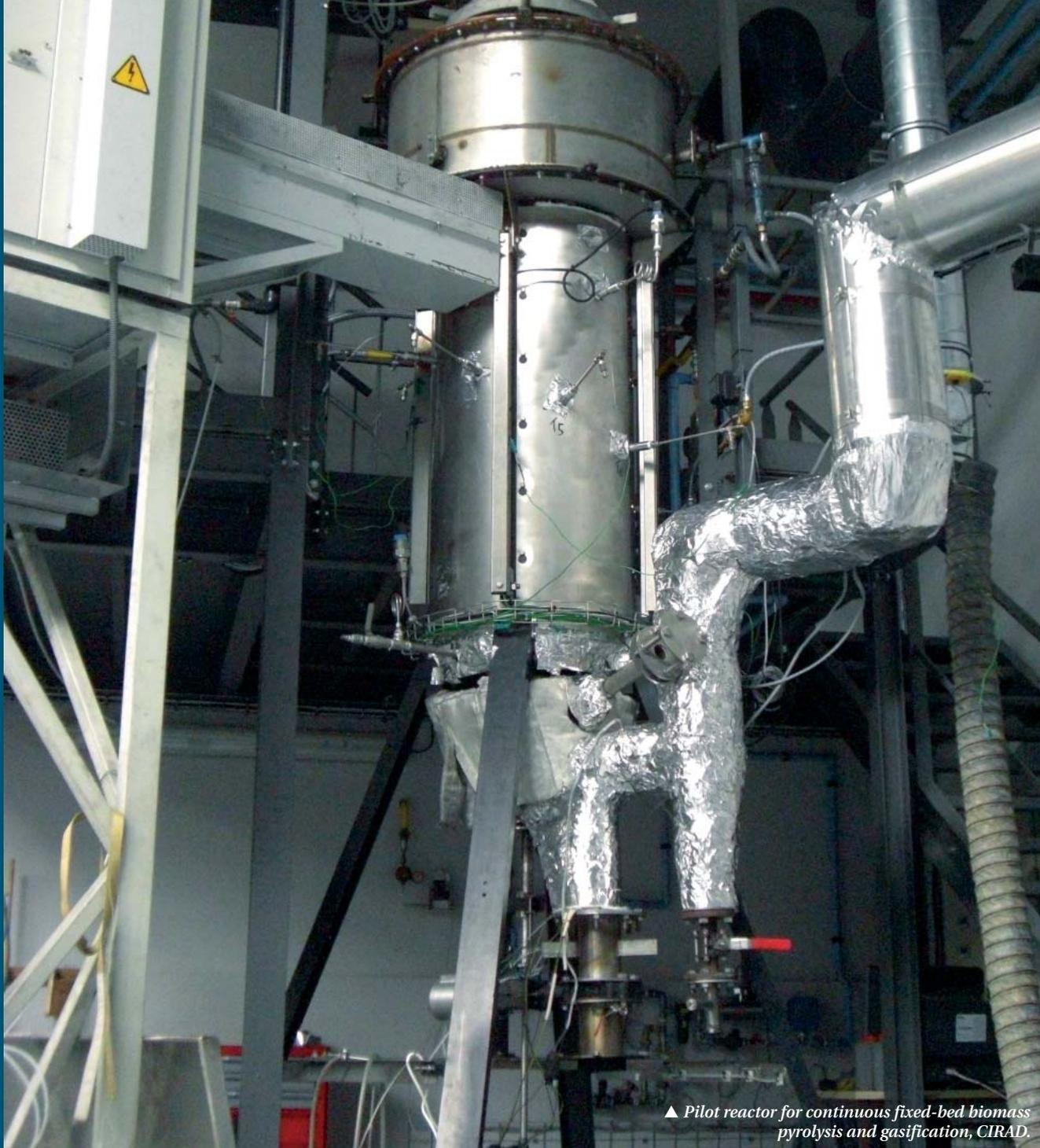
▲ Pilot reactor for continuous fixed-bed biomass pyrolysis and gasification, CIRAD.
