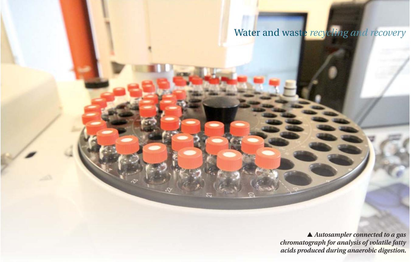
▲ Autosampler connected to a gas chromatograph for analysis of volatile fatty acids produced during anaerobic digestion.
