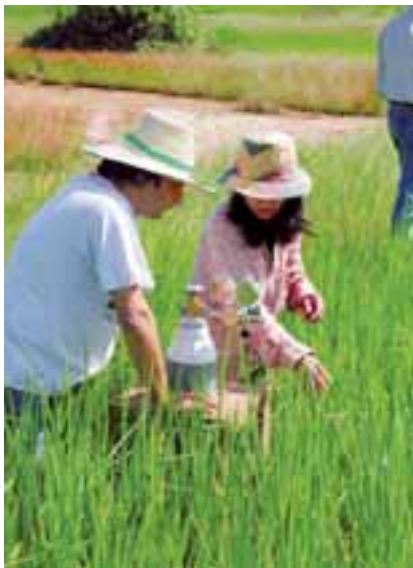
Sampling the soil solution under a nitrogen atmosphere in a rice field in northern Thailand
