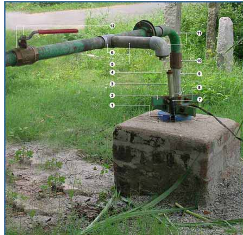
TYPICAL OBSERVATION BOREWELL AND ITS MODIFIED COMPONENTS
